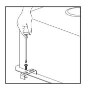
NOTE: the clip is ¾" wide and 2-¾" long. It may be too long in some cases. If so, make a brace of wood or solid surface material, butt it up against the sink, and screw it into the cabinet wall (this must be done on site). Make sure that the screw does not go through to the other side of the cabinet.
