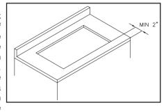
also placed on plywood, as explained for the sink. However, the use of the actual sink ensures a more accurate cutout. Mark the center of the sink on the template. If you use a 5/8" template guide on the router, draw another line 1/16" outside the outline of the sink (this makes room for the template guide). If you use other cutting methods, adapt this accordingly.
