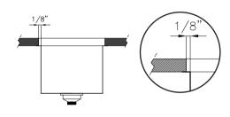
Zero reveal: the cut-out exactly matches the bowl's dimension
